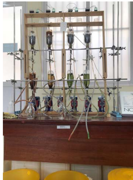
Fig.1. Schema of experiment design for As removal
